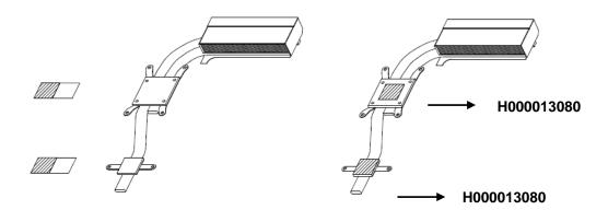
Figure 4-40 Applying new thermal pad
